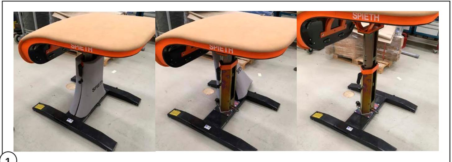
2. Loosen the screws on both the sides of the orange bracket with the Allen key.
